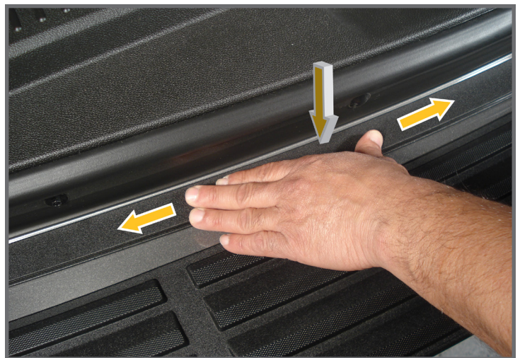
Push down to seat mounting tape, while holding assembly against the front sill of the bumper. Apply pressure against length of assembly to seat mounting tape.
