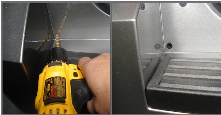
Drill hole using 5/16" bit. Insert supplied 1/4" grommet.
