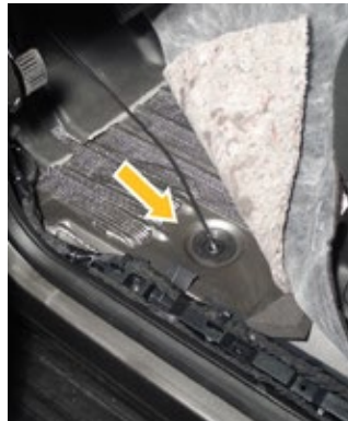
[Left] Factory grommet for wire routing. [Right] Using an awl, create access Passenger side factory grommet. Route wiring to Runner Platform Module [RPM12].
