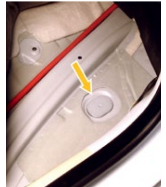
[Left] Driver side factory grommet for wire routing. [Right] Passenger side factory grommet. Route wiring to Runner Platform Module [RPM12].
