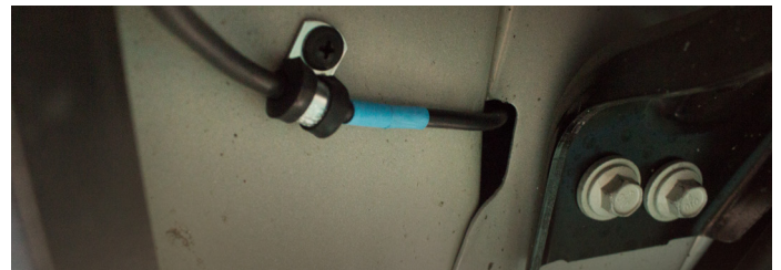
Fasten wire stress-relief clamp to underside of vehicle in a suitable location using self-tapping sheet metal screw.
