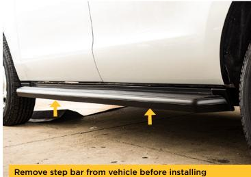
Remove step bar from vehicle before installing Arrows indicate bolts not visibile in photo.
