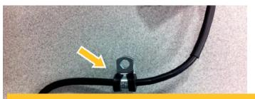
Fasten wire stress-relief clamp to underside of vehicle in a suitable location using self-tapping sheet metal screw.
