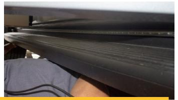
Use another person to assist with remounting step bar to vehicle. Ensure Runner doesn't obstruct door before securing.
