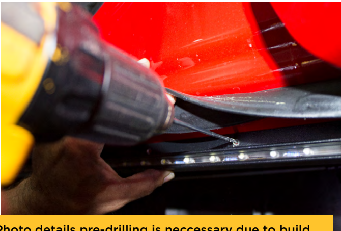
Photo details pre-drilling is necessary due to build of vehicle and the thickness of metal on body frame.
