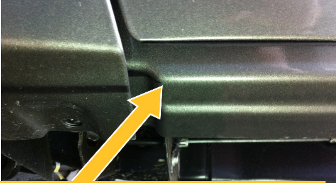
Detail photo illustrates driver front rocker panel. The front of the HG2 Runner assembly aligns with this body line.
