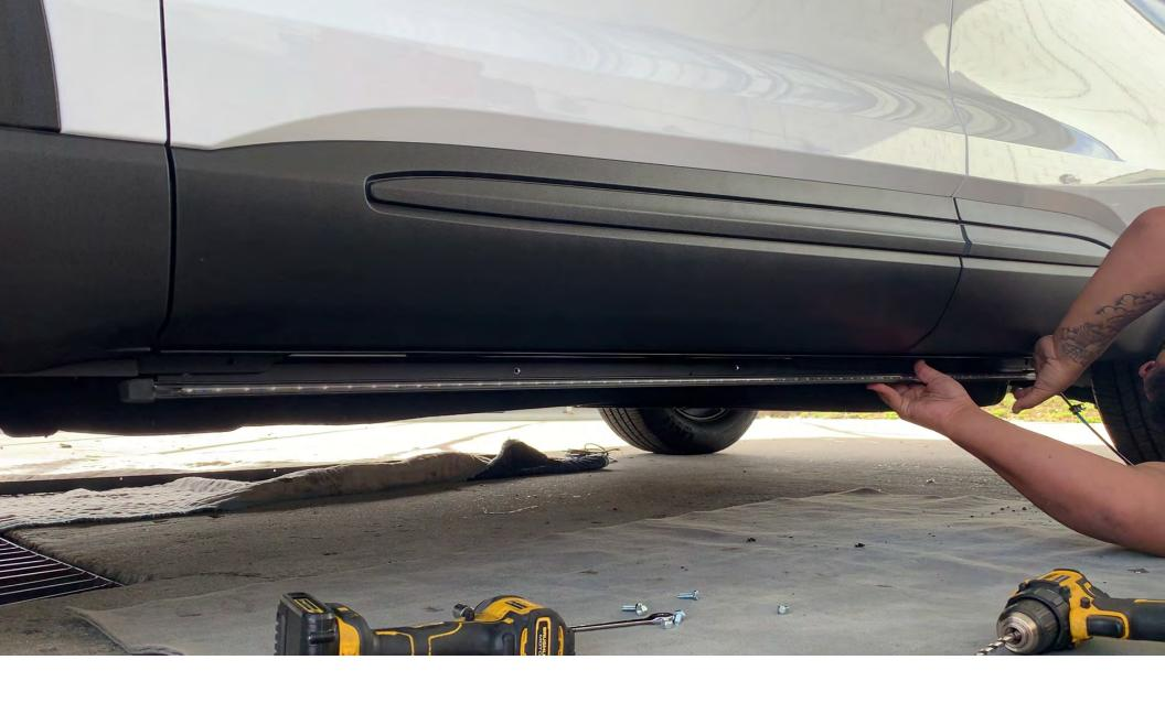
3. Line up the HG2 Siderunner with the holes on the metal tab (pre-drilled holes in HG2 Siderunner will not line up with the metal holes)
