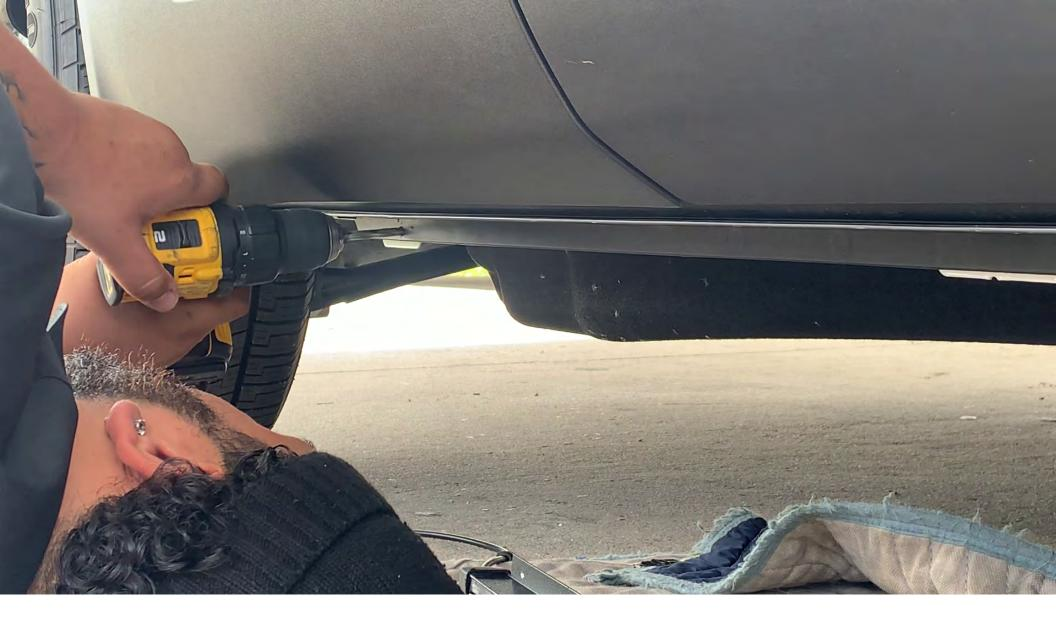
4. Drill holes in plastic piece corresponding to the correct hole in each tab
