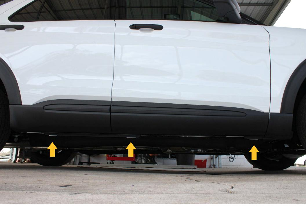
1. Locate tabs under vehicle (Notice: There is a plastic tab in front of a metal tab)
