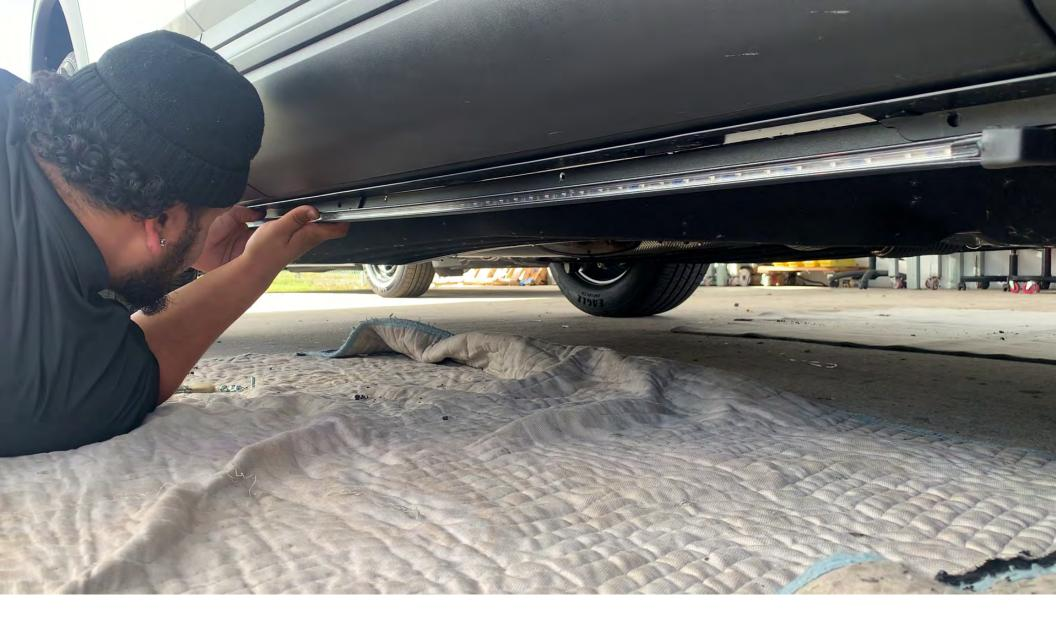
5. Line up and mark the bracket of the HG2 Siderunner to the corresponding hole by placing the HG2 Siderunner in between the plastic and metal piece
