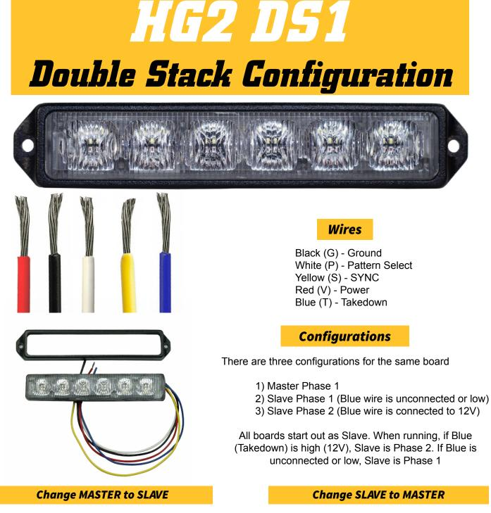
Connect WHITE (Pattern\_Sel) to RED. BLACK to Ground. Apply 12V to RED and WHITE for 5 seconds. Module will flash twice when it becomes a Master. Remove WHITE (Pattern\_ Sel) from RED.
