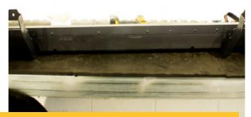
Photo details placement of #8 1/2" screws. Note: Make sure Runner light is tightly secured to step bar.
