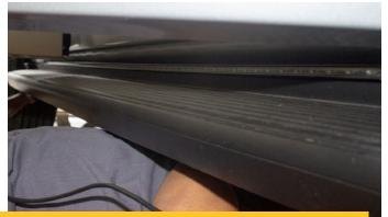
Use another person to assist with remounting step bar to vehicle. Ensure Runner doesn't obstruct door before securing.
