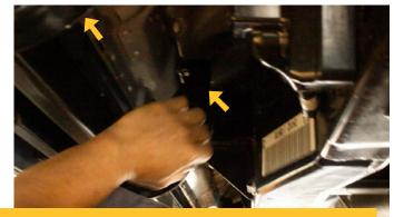
Arrows illustrates locations to secure step bar to underside of vehicle.
