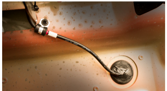
Photo illustrates wiring being fastened into underside of vehicle using wire clamp(included) and sealed inside factory grommet vehicle.
