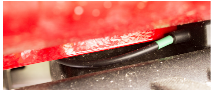
Photo illustrates wiring being routed behind runner assembly and body frame to Route wiring to Runner Platform Module [RPM12].
