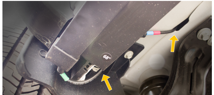
Arrows in photo illustrates factory grommet area and area to route wiring under vehicle to Runner Platform Module [RPM12]
