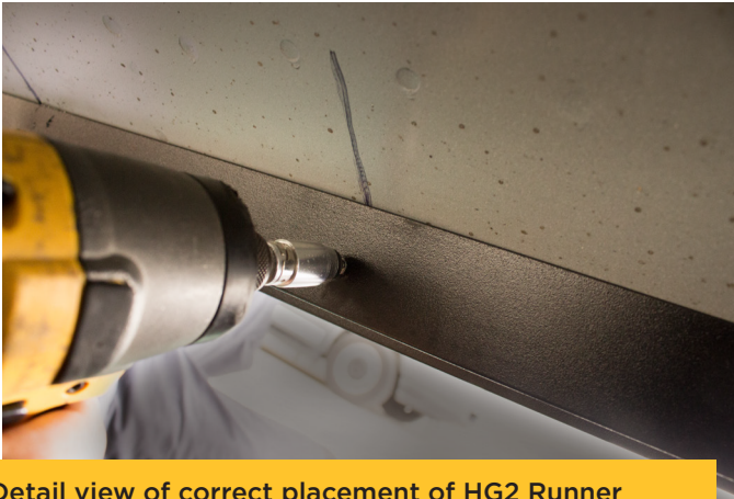
Detail view of correct placement of HG2 Runner assembly. Rear of HG2 Runner assembly butts against rocker panel seam flange.
