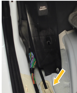
[Left] Driver side factory grommet for wire routing. [Right] Passenger side factory grommet. Route wiring to Runner Platform Module [RPM12].
