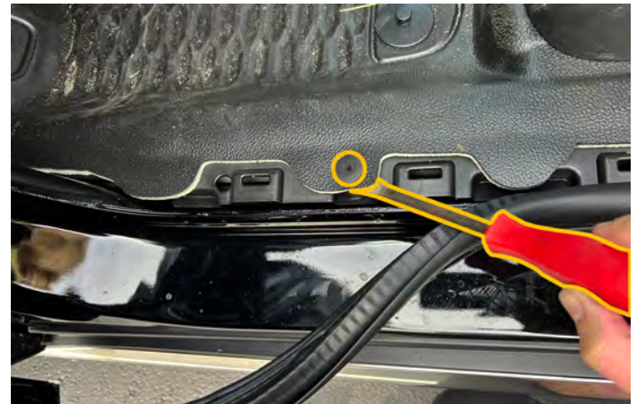
4. Pull out push pin with panel popper.
