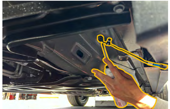
17. Silicon wire hole closed.
