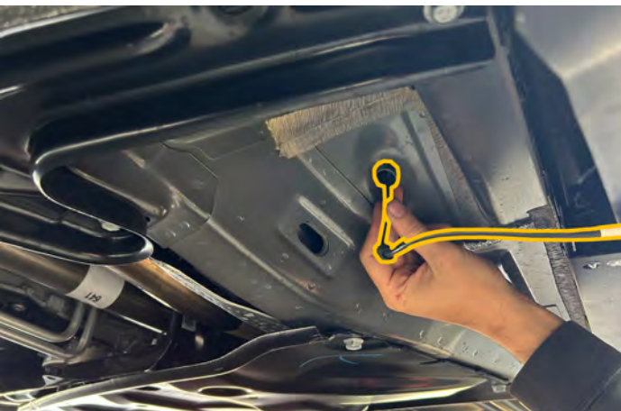
15. Feed wire through hole.
