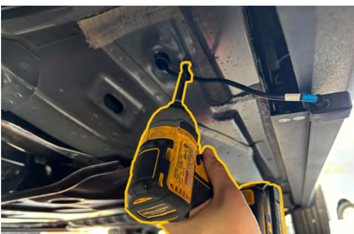
16. Secure wire with provided wire-holder.
