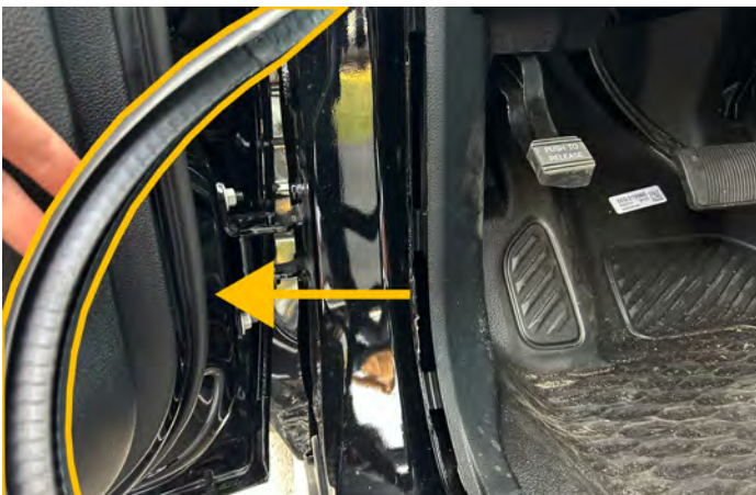
2. Pull weather stripping.
