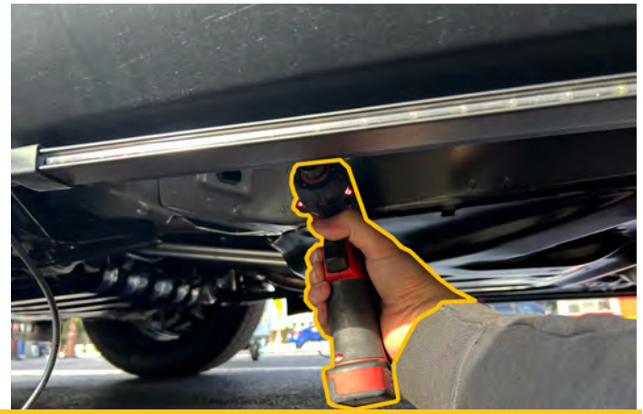
13. Secure in place with three 1/2" self-tappers.
