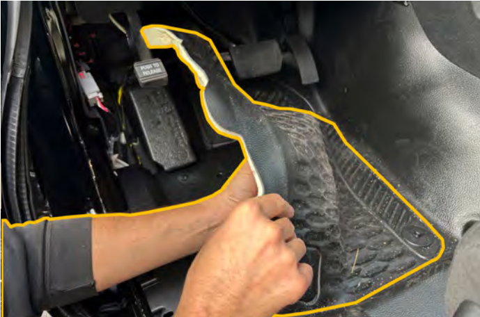
5. Lift carpet and remove footrest dead pedal.
