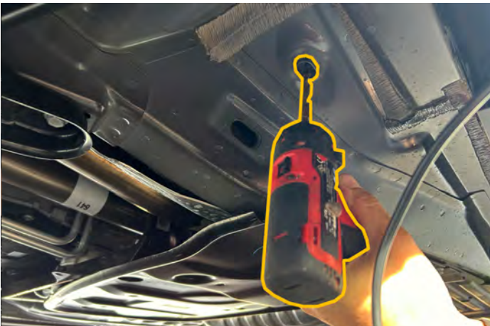
14. Use 5/16" drill bit to drill a whole into plastic plug.
