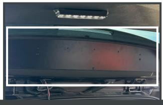
13. Thread the wire loom through the plastic trim panel and trim connector into the body panel. Route the wire to the existing power using the harness or controller.
