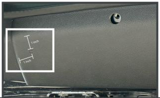
6. Measure 1 inch from the driver's side on the plastic trim and 1 inch from the curve. Drill 1 additional 5/16 hole for the wiring harness to run under the plastic trim. Exercise caution to avoid drilling through the existing harness; drill pieces separately.
