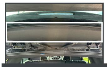
1. Disassemble by pulling down the rear visor trim. Position the template guide face up on the plastic trim.
