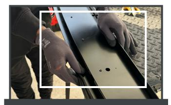
7. Attach the rubber glass seal/flashback gasket to the light assembly.
