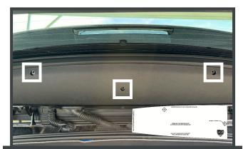
2. Align the driver's side short edge with the mark and drill two holes using a 5/8 bit. Flip the template, align the short edge to the marked location on the passenger side, and drill a third hole.
