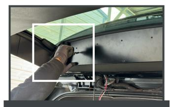
11. Insert the bolt on the driver's side and hand-tighten.
