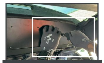
12. Proceed to the next bolt on the passenger side and hand-tighten.
