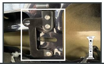
3. After removing the trim, insert the supplied Driver's Side Bracket template into the space, aligning with the punched hole. Use the template guide for alignment. Drill three 5/16 holes and attach the bracket with supplied screws.
