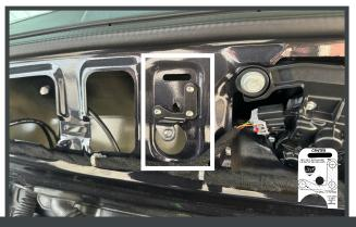
4. Insert the provided Center Bracket template into the space, aligning with punched holes and curve. Utilize the template guide for alignment. Drill three 5/16 holes and secure the bracket with supplied screws.
