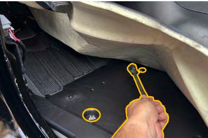
6. Remove two 10 mL nuts (this will loosen the plastic floorboard).
