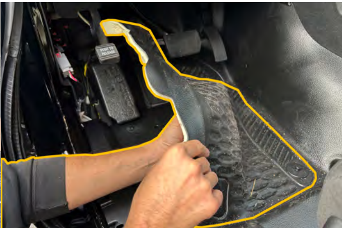
5. Lift carpet and remove footrest dead pedal.
