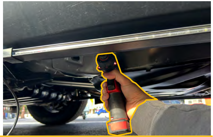
13. Secure in place with three 1/2" self-tappers.
