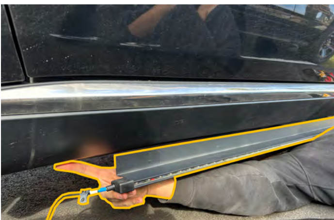
12. Line up the HG2 Side Runner to the edge of L-bracket and pre-drill front holes.
