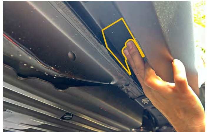
8. Make sure brackets are flushed to corner.
