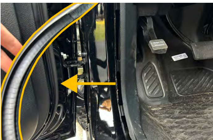
2. Pull weather stripping.
