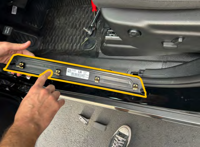
1. Remove plastic kick panel from the seam on the inside of the car.
