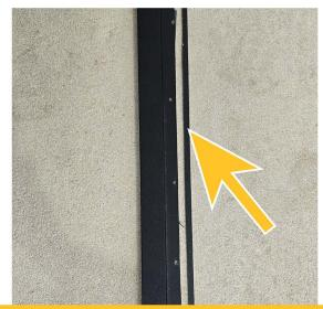
1. Cut 1/4 to 1/2 inch off to make flush to vehicle.
