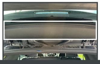
1. Disassemble by pulling down the rear visor trim. Position the template guide face up on the plastic trim.
