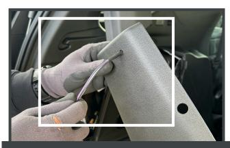
Thread the wire loom through the plastic trim panel and trim connector into the body panel. Route the wire to the existing power through the harness or controller.
