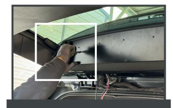
11. Insert the bolt on the driver's side and hand-tighten.
