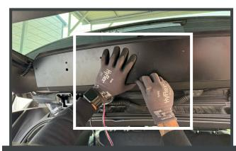
Use the provided 3 bolts for light installation. The longer bolt is for center installation; place it first to hang the light. Hand tighten only—avoid power tools and over-tightening.
