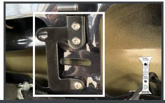
After removing the trim, insert the supplied Driver's Side Bracket template into the space, aligning with the punched hole. Use the template guide for alignment. Drill three 5/16 holes and attach the bracket with supplied screws.
