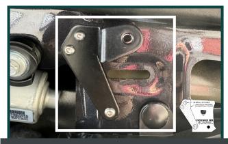
Insert the provided Passenger Bracket template into the space, aligning with punched holes. Utilize the template guide for alignment. Drill three 5/16 holes and secure the bracket with supplied screws.
