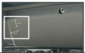
6. Measure 1 inch from the driver's side on the plastic trim and 1 inch from the curve. Drill 1 additional 5/16 hole for the wiring harness to run under the plastic trim. Exercise caution to avoid drilling through the existing harness; drill pieces separately.
