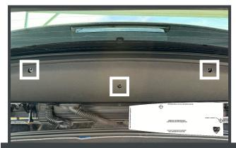
2. Align the driver's side short edge with the mark and drill two holes using a 5/8 bit. Flip the template, align the short edge to the marked location on the passenger side, and drill a third hole.
